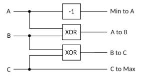
An XOR logic gate is very simple: its output is equal to 1 only if one of the inputs is 1. In all other cases, either both are 0, or both are 1, the output is 0.
