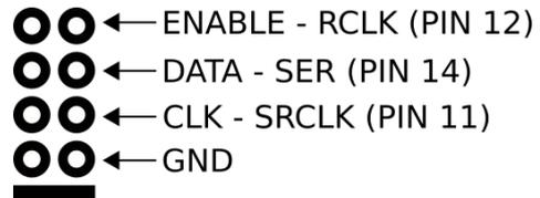
*Here the extension connector. With name of each line, the corresponding name of the IC, with the PIN number.*
