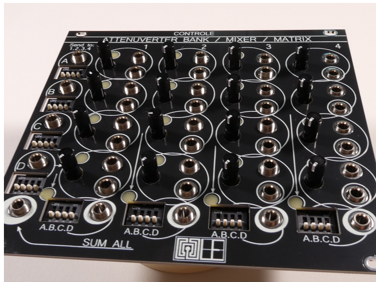
9mm trimmer pots, that doesn't need knobs.
